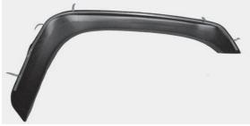
Peel about 2" of the red liner away from one end of the double sided adhesive tape. Pulling the red liner free attach the flare to the fender with firm and even pressure to ensure adhesion.
