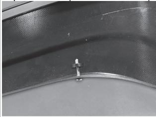
If the factory screws interfere with the fitting without using the plastic washers, you may remove the factory screws and attach the fender without using the plastic washers. Do not wash the vehicle for 24 hours.
