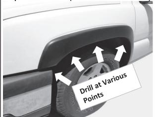
Using a 1/8" diameter drill bit or the provided self tapping screws, attach the flare at the various points.
