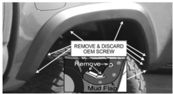
Remove 3 existing screws from the mud flap, save screws for reinstallation. **Remove the factory mud guard.** Remove 7 factory screws and pulling the flare away.
