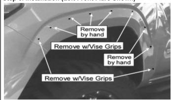
Remove 6 factory clips by hand on the fender. Remove 3 factory clip with vise grips on the fender, as shown.
