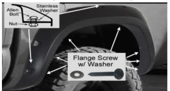
Use hex key to tighten the allen bolt & nut firmly on every pocket of the fender flare, shown as top. **DO NOT OVER TIGHTEN!** Place the flare on fender in right position. Apply 7 supplied Flange screws with washers through the flare & into the factory holes on the wheel well. Ensure the flare is on the proper position, tighten all screws.
