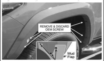
Remove 3 existing screws from the mud flap, save screws for reinstallation. Remove the factory mud guard. Remove 5 factory screws and pulling the flare away.
