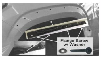
Ensure you have the right inner bracket & know the way to install. Apply 2 U-Clip over 2 holes, as shown. Apply 3 supplied Flange screws with washer through three holes in the bracket, and into the factory holes on the wheel well.
