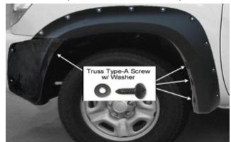
Install 4 supplied truss screws (20mm) into factory holes. (see illustration) Use inculded self tapping screws for extra secure on the bumper piece. Tighten all screws.
