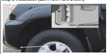
Remove 2 factory screws from the underneath of the factory bumper cover, pull down the bumper cover and splash shield, as bottom right illustration, save screws for reinstallation. Remove 7 factory plastic clips from the inside of the factory bumper cover, as top right illustration. Pull away the factory flare (bumper piece/small part) from vehicle.
