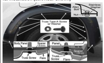
Use hex key to tight allen bolt & nut firmly on every pocket of the fender flare, shown as top. **DO NOT OVER TIGHTEN!** Install 8 supplied truss screw (20mm) into factory holes. (see illustration) Install supplied truss screw (20mm) through spacer (6.5mm) into factory hole on the bottom of front end, as left shown. Install supplied truss screw (50mm) through spacer (19mm) into factory hole on the bottom of rear end, as right shown.
