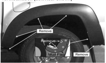
Remove 3 existing screws from the mud flap, save screws for reinstallation and discard mud flap. (see illustration) Remove 5 factory screws as shown. Pull away the factory flare from the vehicle.
