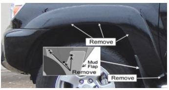
Remove 3 existing screws from the mud flap, save screws for reinstallation. (see illustration) Remove 3 factory screws on the top of the flare lip & 1 screw from the bottom as shown, save screws for reinstallation. Pull away the factory flare (large part) from the vehicle.
