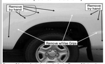
Remove 7 factory clips by hand on the fender. Remove 3 factory clips with vise grips on the fender, as shown.
