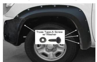
Reinstall 4 factory screws. Use 2 inculded self tapping screws for extra secure on the bumper piece, as top shown. Install supplied truss screw (50mm) through spacer (26mm) intofactory hole on the bottom of bumper piece.
