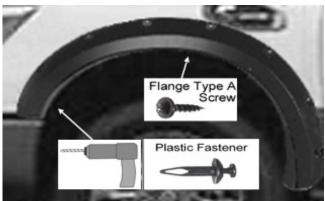
Apply one Flange Screw through inner piece, into U-Clip and secure it to the vehicle on the uppermost hole, as shown. Push the front fender flare to ensure it contact with the fender well, drill a 1/4" hole through the hole on the flare into the wheel well. Secure the flare with a plastic fastener into the hole.
