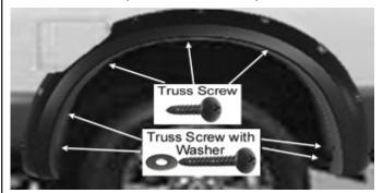
Secure the flare with three Truss Type screws into the long clip. Apply four Truss Type-A Screws through the flare into the factory holes. Tighten all screws.
