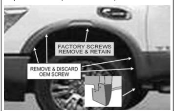
Remove five existing factory screws, save one screw on top center for reinstallation, remove the flare, as shown. Remove factory mud flaps if installed.
