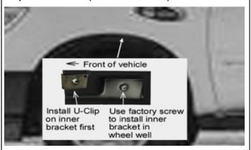
Ensure to have the right inner bracket & knowing the way to install. Install a U-Clip over the hole on the inner bracket first. Install a factory screw through bracket and into factory uppermost hole on the fender wheel well.
