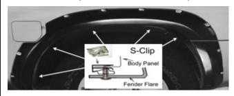
Apply 5 S-Clip over 5 location and secure it with 5 machine screws, as shown in illustration. (**Do not fully tighten screws**) Line up the flare properly and hold the flare firmly, tighten all screws, start from right side toward the access door.
