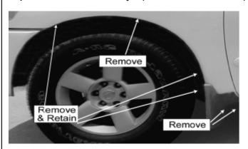
With Mud Flap- Remove existing screws & 1 extra screw above. save screws for reinstallation. (see illustration) Without Mud Flap- Remove 2 factory screws on the side, Remove 1 factory screw located at most front of fender, just above the bumper, save screw for reinstallation. Remove 1 factory screw located at most top of fender.
