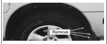
With Mud Flap Remove existing screws & 1 extra screw above. (see illustration)
