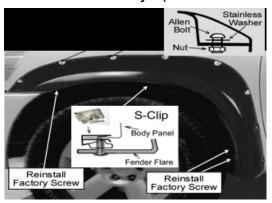
Use hex key to tighten allen bolt & nylon nut firmly on every pocket of the fender flares. DO NOT OVER TIGHTEN! Apply 2 S-Clip over 2 location and secure it with 2 machine screws.(Do not fully tighten screws) (see illustration) Line up the 3 holes in flare with factory holes and hold the flare firmly, reinstall 3 factory screws into the holes that were previously removed. (see illustration) Tighten the screws on
