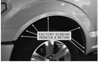
Remove the five existing factory screws with proper wrench. Remove the two rear most existing factory screws with proper wrench and save for reinstallation later.
