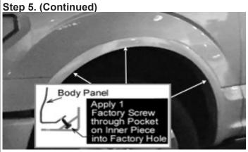
Ensure to have the right inner piece and knowing the way to install first, and line up the holes on inner piece and 3 uppermost factory holes. Use the proper wrench to reinstall 3 factory screws, through the holes on the inner piece into the factory holes.
