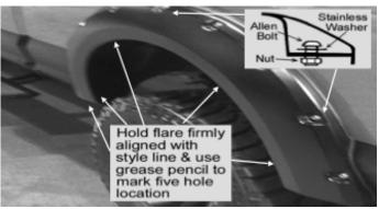
Use Torx Bit to tighten allen bold & nylon nut firmly on every pocket of hte fender flares. **DO NOT OVER TIGHTEN!** Place the flare on the vehicle with best position, mark the five hole locations into the vehicle.
