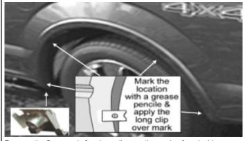
Remove the flare, apply four long clip over the marks, from inside toward to outside, as shown. Install a S-Clip on the lower front of the rear wheel well, align with the mark made in previous step.
