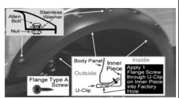
Use Torx Bit to tight allen bolt & nylon nut firmly on every pocket of the fender flares. **DO NOT OVER TIGHTEN!** Apply 3 Flage Screws through inner piece, into U-Clip and secure it to the vehicle on the uppermost holes, as shown.
