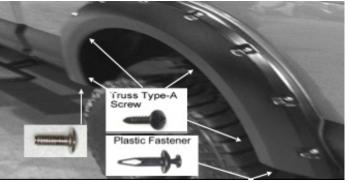
Secure the flare with four Truss Type screws into the long clip, start the two screws on the two topmost holes, as top shown. Apply 1 Truss Machine Screw into the installed S-Clip. Apply one Plastic Fastener into flare and through the same factory hole in step 9.
