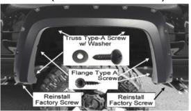
Install 3 supplied truss type A screws into the factory holes. Re-install the 2 factory screws underside, removed in step 11. Install 3 supplied flange type A screws into the holes drilled in step 13.
