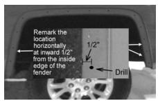
Remark the 3 locations (marked in step 12) horizontally inward 1/2" from the inside edge of the fender. Drill a hole on the marked locations through sheet metal with a 3/32" drill bit. (use a floor jack on the rear hitch to raise the truck bed for easier drilling)
