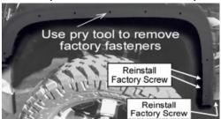
Pull the lower grip part to remove the factory flare from vehicle. Use pry tool to remove any remaining factory fasteners. **FOR MODELS WITH FACTORY MUDFLAP:** Re-install the upper two fasteners (removed in step 5-2). Use a 1/2" socket to re-install fastener (removed in step 6-3) from the rear underside of factory wheel arch molding.
