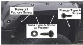
Install 4 supplied truss type A screws into the factory holes. Re-install the factory screw, removed in step 6-1. Install 1 supplied flange type A screw into the hole drilled.
