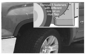
Make sure the front tire has been turned to outward for easy installation. FOR MODELS WITH FACTORY MUDFLAP: Remove 5 mud flap fasteners with T-30, T-15 torx bit & screw driver. Save the upper two fasteners for re-install in step 7.
