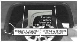
Use a 10mm socket to remove the lower 2 screws. Use T-15 torx bit to remove the others 3 fastener. Use pry tool to remove any remaining factory fasteners. Pull the lower grip part to remove the factory flare from vehicle.
