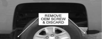
Remove and discard the existing screws on the mud guards with a Torx Bit (T-15).
