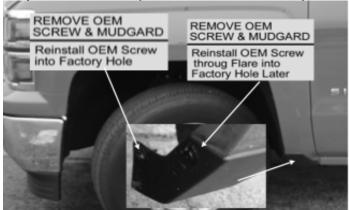
Make sure the front tire has been turned outward for easy installation. Remove 2 existing screws on the mud guard with a Torx Bit (T-15). Remove the mud guard. Reinstall the lower screw into the factory hole right away. Retain the upper screw for next step.
